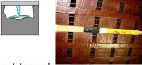
Figure 8: PD pattern for slot discharge at machine bars
